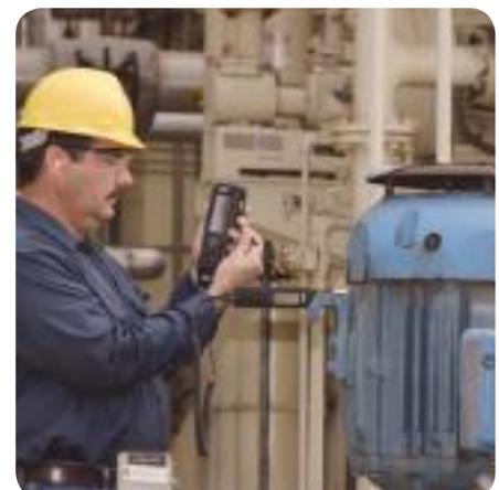
SKF Machine Condition Detector Pro IS CMVL 3600-IS
