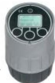
*Test cell: digital analysis of Total Base Number and water in oil*
