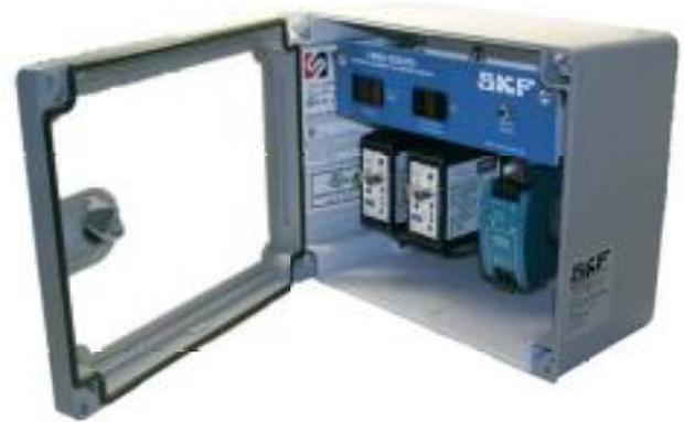
The system is a pre-wired, turnkey package with power supply and bright LED displays. The power supply accepts 110 or 220 VAC, 50 or 60 Hz. They are available in either an Imperial or Metric configuration. The standard enclosure is NEMA 4X fiberglass; powder coated steel and stainless steel enclosures are available.
