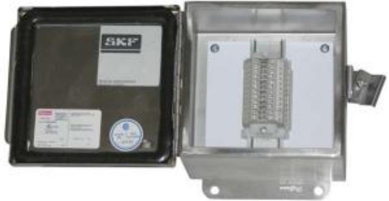
The CMSS 265 series termination junction boxes are multiple channel connecting centers for terminating the outputs of accelerometers or other transducer field wiring. Crew clamp, DIN-rail mounted terminals (three inputs per channel, usually signal, common and shield) are provided for the intermediate termination of accelerometers, proximity probes, speed sensors, RTDs and other transducers.
