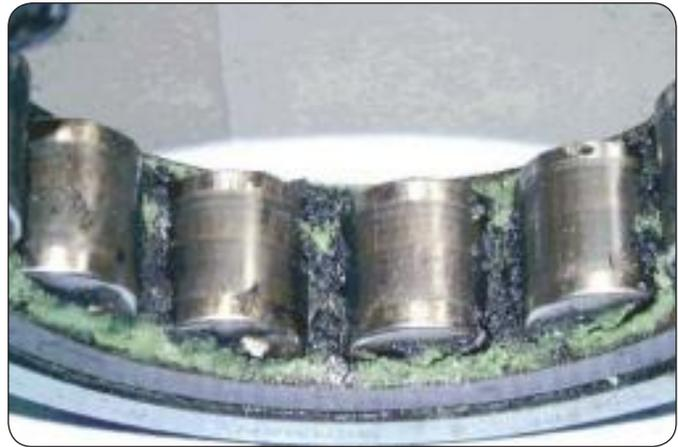
*Lubricant degradation caused by electrical discharge currents.*
