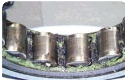
Lubricant degradation caused by electrical discharge currents.
