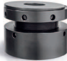
Extended SKF Vibracon chocks or additional bottom rings For installations with larger gaps between machine foot and foundation. The maximum extended height should not exceed the diameter of the chock.
