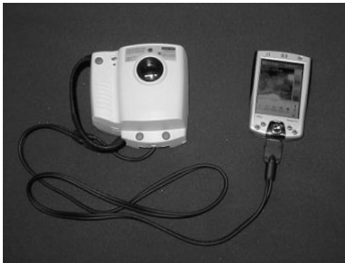
Figure 3: The TMTI 300 Thermal Imager connected to a 'Pocket PC', configured for two handed operation
